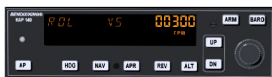
Figure 10.6: Autopilot after engaging
