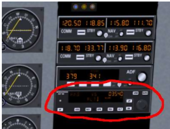
Figure 9.10: The C172 Autopilot
